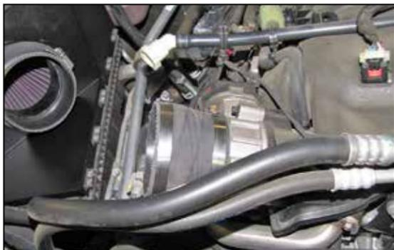
16. Install the provided step coupler (08497) onto the throttle body and secure with the provided hose clamps.
