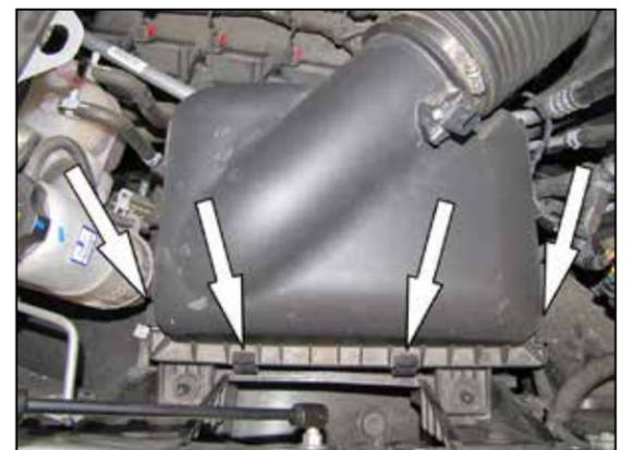
6. Release the four locking tabs securing the air filter housing lid and then remove the housing lid and factory intake tube from the vehicle. Remove the factory air filter.
