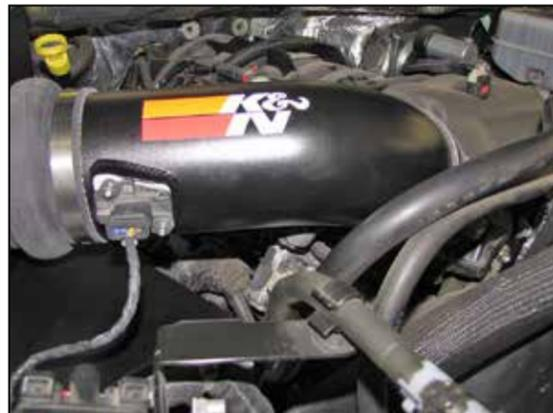
19. Reconnect the humidity sensor and inlet air temperature sensor electrical connections.
