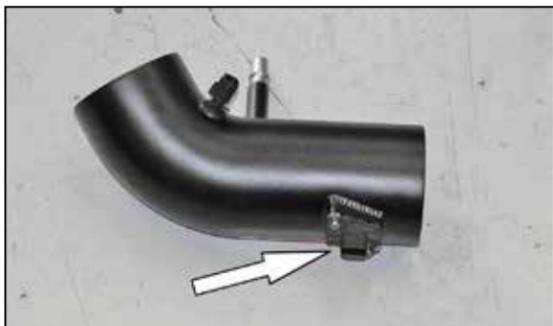
14. Install the humidity sensor into the K&N® intake tube and secure with the provided hardware.
