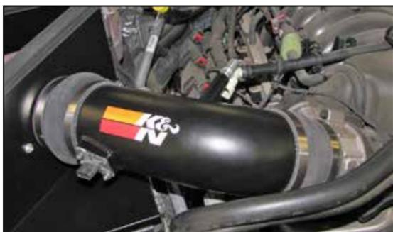
17. Install the K&N® intake tube into the hump coupler and then into the step coupler, then adjust the tube for best fit and secure with the provided hose clamps.
